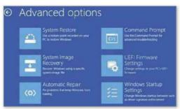
Click Automatic Repair in Windows 8's 'Advanced options' to fix the infinite startup loop.
