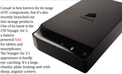
As with any mobile NAS device, files are copied onto the Voyager 2 via USB 3.0 from your computer, and then accessed from your mobile device over a Wi-Fi network. The Voyager 2's fast USB3 performance was pretty much what we'd expect. We had no trouble wirelessly streaming three HD video files simultaneously. Impressively, we were able to wander 20 feet from the Voyager 2's built-in 802.11n hotspot and up a flight of stairs before we lost the wireless signal.
